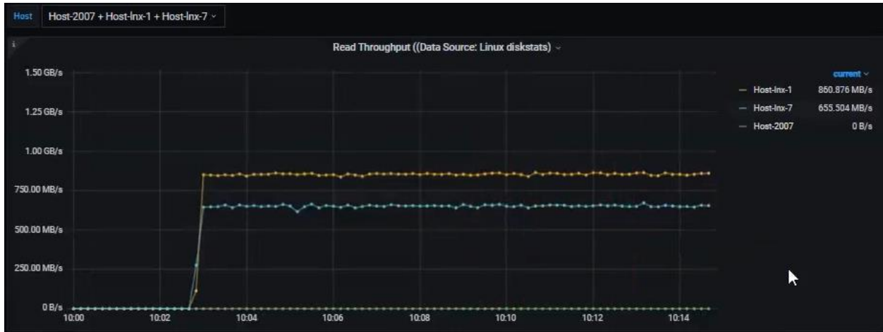
Throughput for the Inx-1 and Inx-7 without any SAN congestion.
