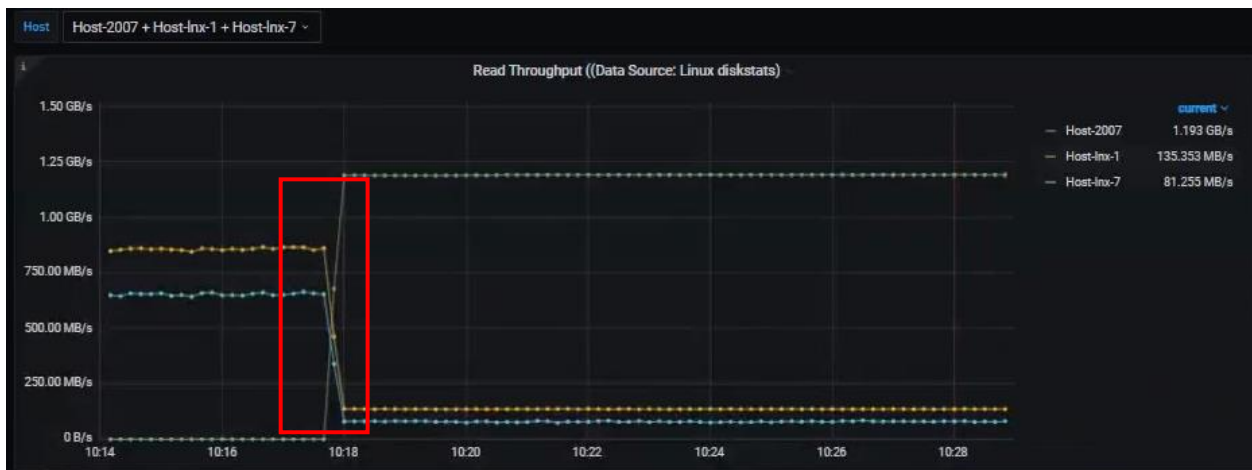
Traffic increased for the Host2007 and declined for Host Inx-7 and Host Inx-1, causing a slow-drain congestion event.
