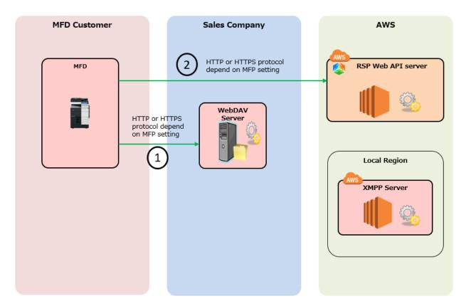
The MFP stores setting data and log files using the WebDAV server at the business server via HTTP/HTTPS, and acknowledgment is made from the MFP to the Remote Service Platform over HTTP/HTTPS to request the download of the result. The WebDAV server grabs the file from the Amazon Cloud (AWS) to the MFP and reboots.
