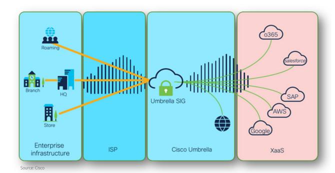
We employed a typical enterprise network connectivity pattern above. Each workstation was directly connected to the internet first without Umbrella, then with Umbrella with no policies set, and then with Umbrella with all security features and full inspection enabled. Within each application, we tested the performance associated with file downloads, page loads, and latency – for 10 minutes.
