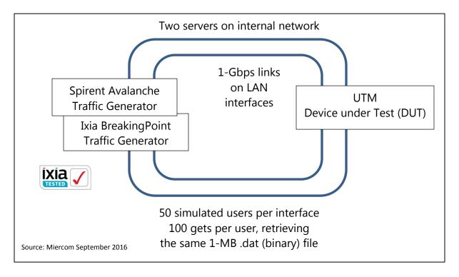
As the diagram shows, *Spirent Avalanche* clients were external and connected to two LAN ports of the Device under Test (DUT). *Avalanche* servers were on the protected internal network and likewise connected through LAN ports of the DUT.
