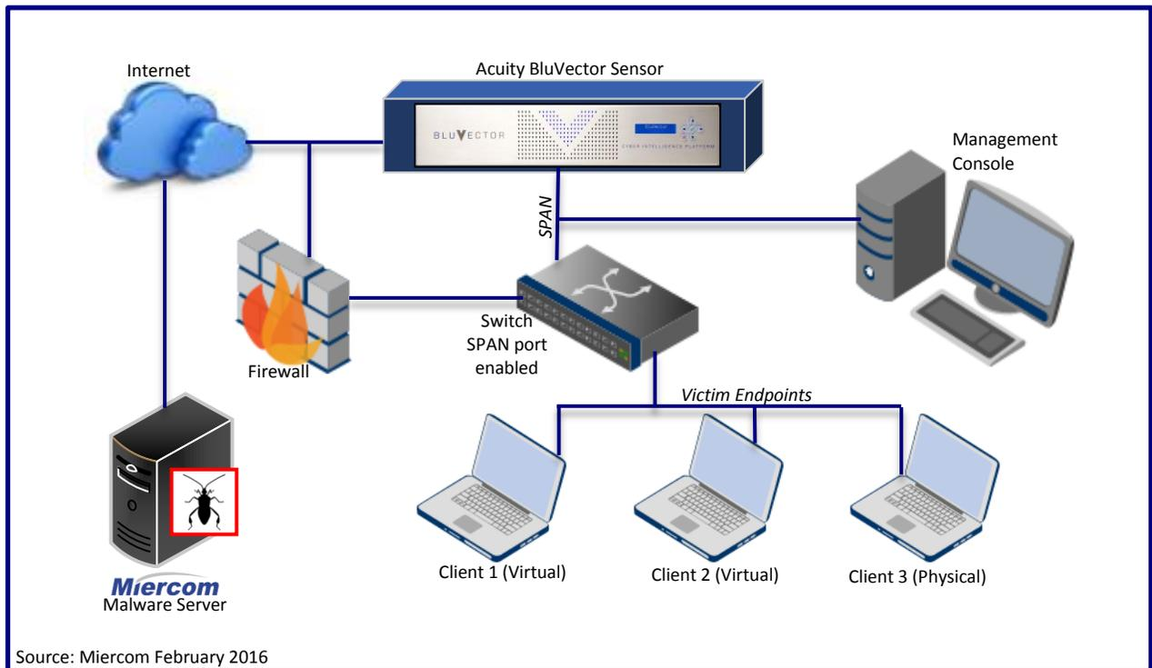
The device under test was the Acuity Solutions BluVector Sensor. It was connected to a Dell N2024P 24-port 1GB switch. Three victims were also connected to the switch; one physical Windows 7 computer and two virtual Windows 7 computers.
