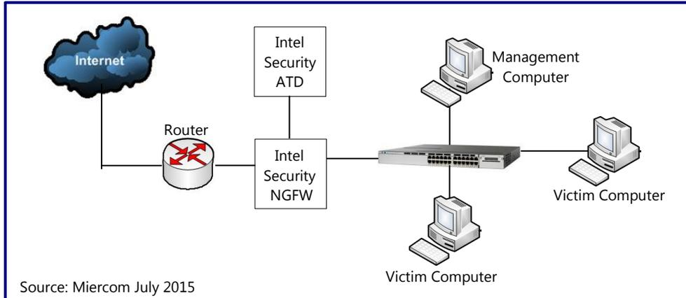
The test bed is structured so the security package under test, in this case two appliances, acts as a logical intermediary between the victim and attacking machines.
