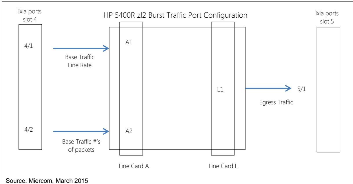
The same set of tests was then applied in the same manner to the HP 5400R zL2 switch (see above diagram). One port (Port 1 on the 10G line card in slot A) carried the Base Traffic Flow at line rate to the output port (Port 1 on the 10G line card in slot L), while a second port on the line card A carries the burst flow of a specific number of packets.
