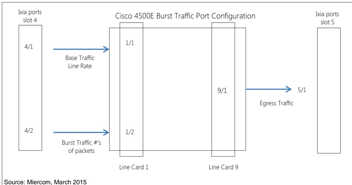
The Ixia test system delivered a 10-Gbps, Layer-2 traffic flow in one direction to Port 1 on the 10GE line card in slot 1 of the Cisco 4500E switch. This line-rate "Base Traffic Flow" was forwarded to output on Port 1 on the 10GE line card in slot 9, and delivered back out to the Ixia traffic generator. This traffic flow, which changed for each test packet size, would fully load the outbound channel of Port 9/1. The Ixia would confirm that there was no packet loss.
