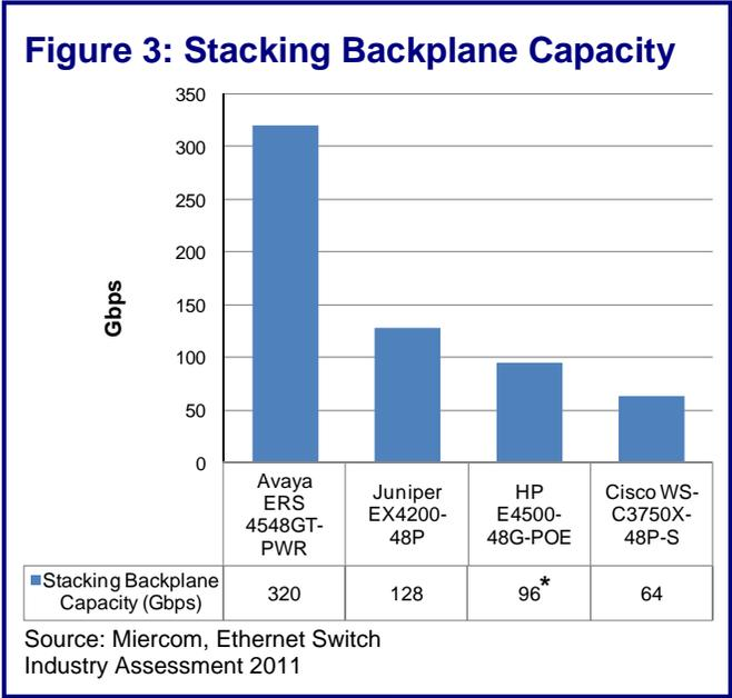
Backplane and switch fabric capacity of each edge switch tested. \* 96Gbps is the stacking capacity for the HP E5500-48G-PoE switch, a larger capacity model in the same switch family. Capacity of the HP E4500 model is not published.
