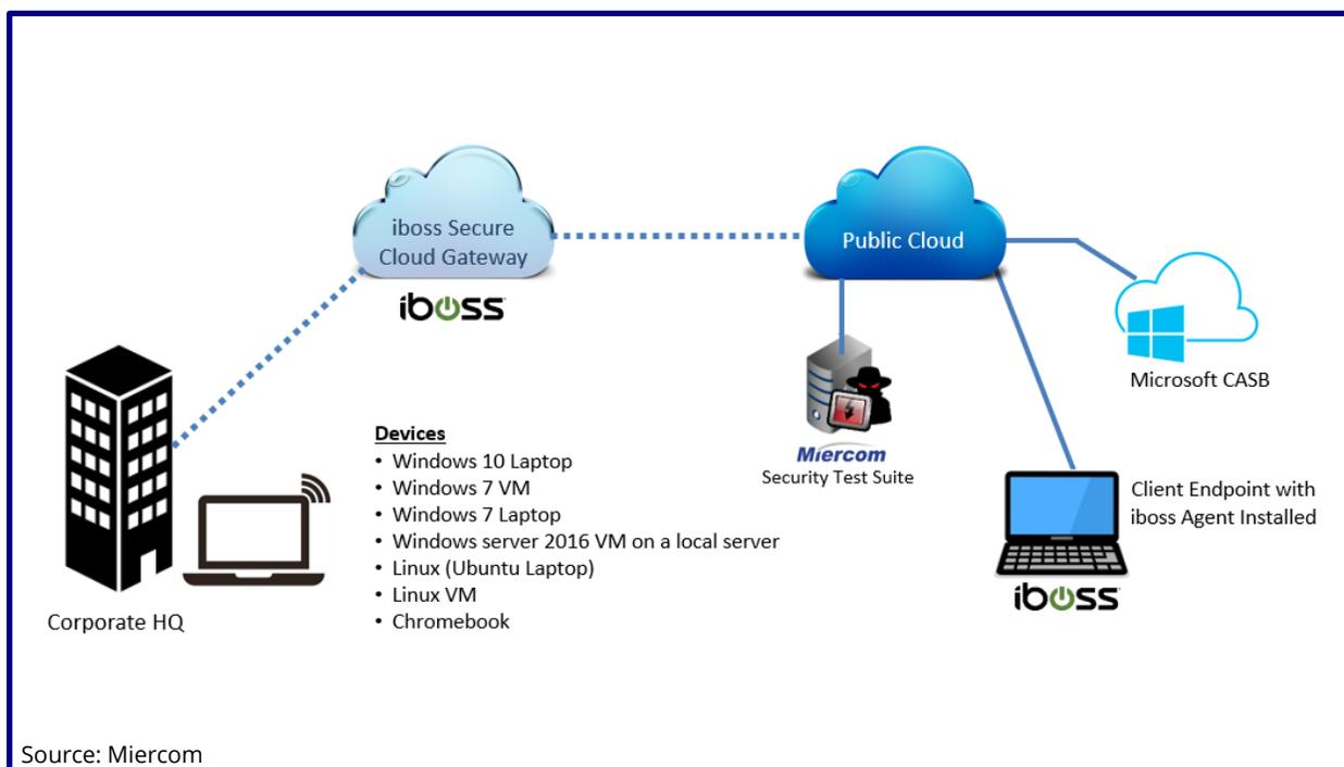
*The test bed above depicts the setup used to simulate an enterprise infrastructure with the iboss Secure Cloud Gateway platform deployed. The SUT was deployed in the cloud, between the corporate headquarters' network with its connected devices and the public cloud with the iboss agent installed. The Miercom Security Testing suite was connected to the public cloud, along with the Microsoft Cloud Access Security Broker (CASB) solution.*
