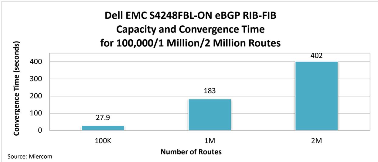
*The Dell EMC S4248FBL-ON switch eBGP convergence with 100,000 (100K) routes took 27.9 seconds to converge. The switch was then tested for the scalability of up to 2 million (2M) routes. These routes were successfully processed with forwarding data in 402 seconds.*
