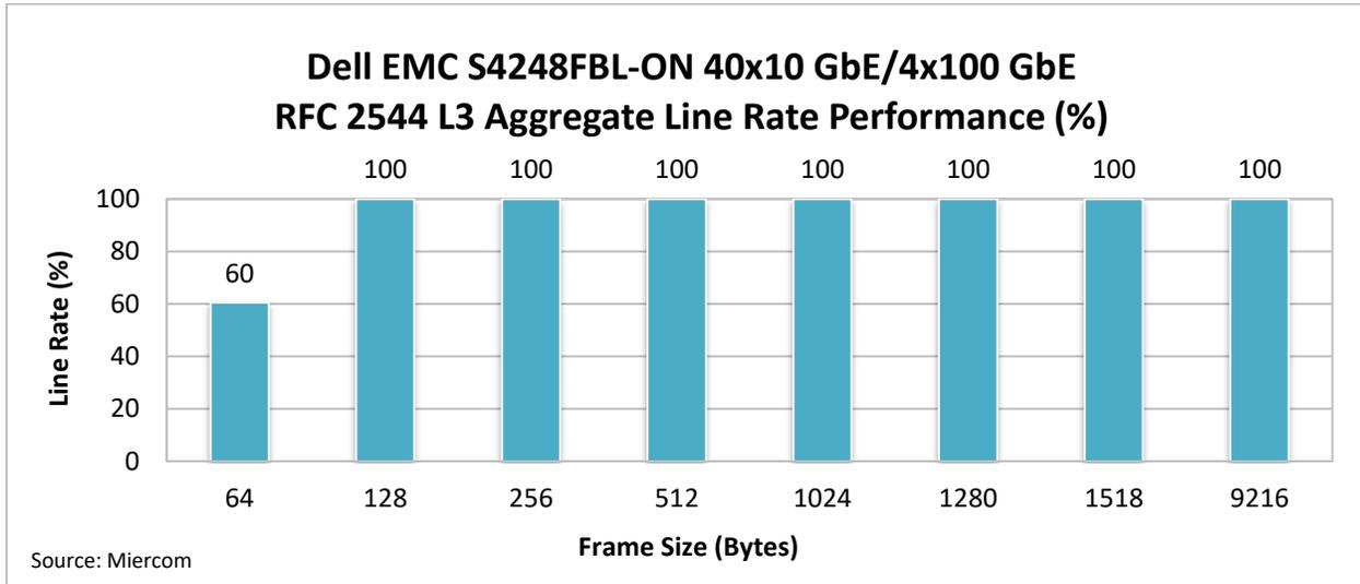
After Layer 2 traffic testing, throughput was measured for Layer 3 traffic. The test-load generator forwarded and received 800 Gbps of traffic through each directly connected 10/100 GbE port using 64, 128, 256, 512, 1024, 1280, 1518 and 9216-byte frame sizes. The Dell EMC S4248FBL-ON switch forwards Layer 3 packets at 100 percent line rate for all frame sizes above 64 bytes, achieving a maximum forwarding rate of 720 Mpps. The switch can forward frames at wire-speed without any loss.
