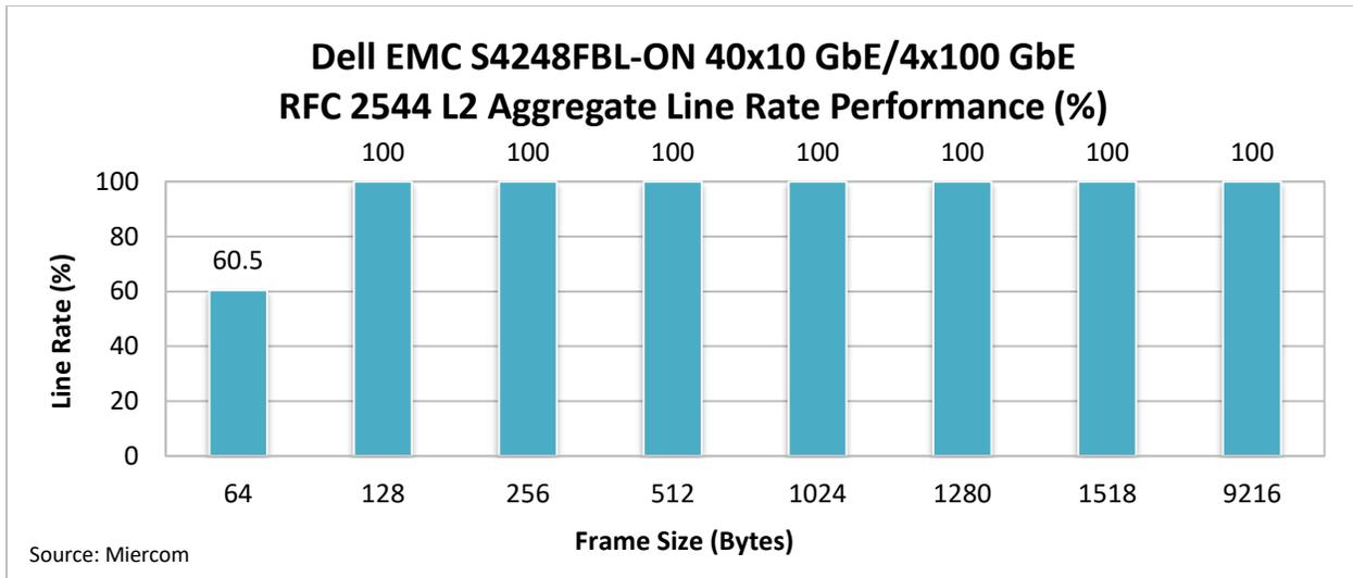
The test-load generator forwarded and received 800 Gigabits per second (Gbps) of traffic through each directly connected 10 and 100 GbE port pairs. The test was conducted for a range of frame sizes including 64, 128, 256, 512, 1024, 1280, 1518 and 9216 bytes. The Dell EMC S4248FBL-ON switch forwards Layer 2 frames at 100 percent line rate for all frame sizes above 64 bytes, achieving a maximum forwarding rate of 720 Mpps. The switch can forward frames at wire-speed without any loss.
