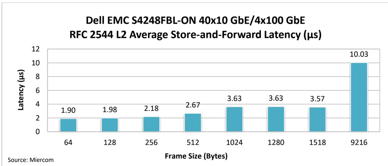
Average latency of the Dell EMC S4248FBL-ON switch was as low as 1.9 microseconds for 64-byte frames. As expected, larger frames typically require more processing, resulting in more latency but remained under 10.03 microseconds. The maximum latency by packet size rose from 1.9 to 10.03 microseconds. For these latency measurements, the switch was subjected to a 100-percent traffic load of Layer 3 IPv4 unicast traffic on all 44 ports. Latency measurements were done in accordance with RFC 2544.
