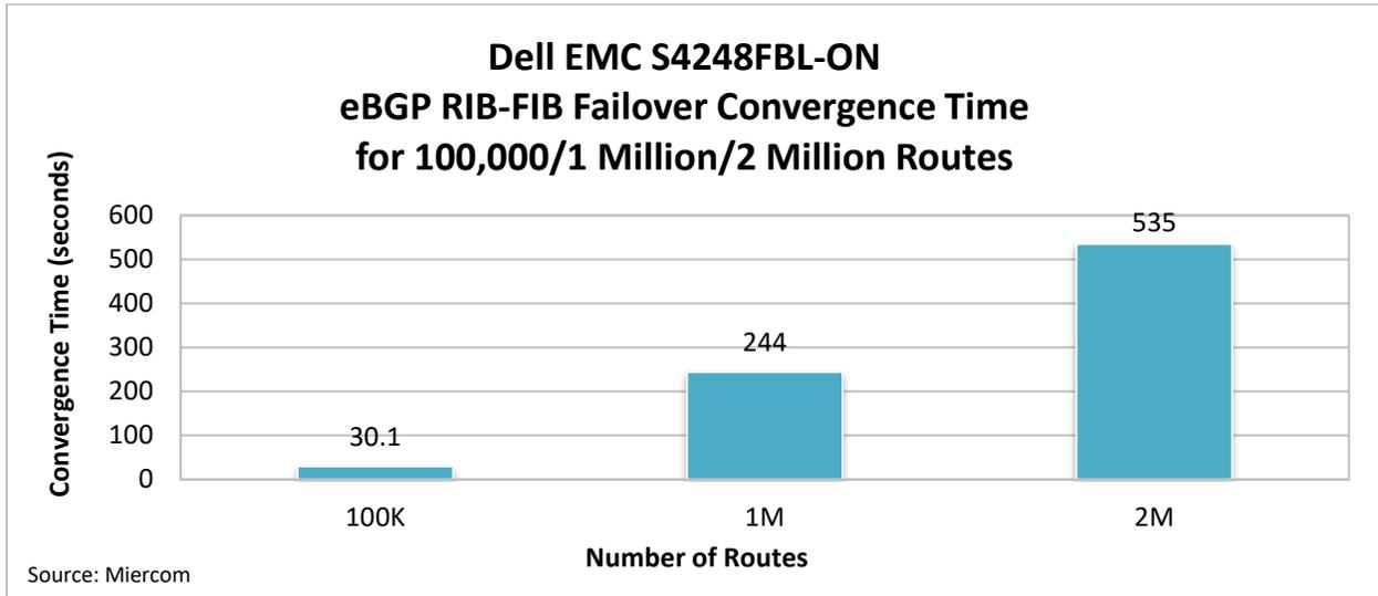
*The Dell EMC S4248FBL-ON switch eBGP failover convergence of 100,000 (100K) routes took 30.1 seconds to complete. The switch was then tested for the scalability of up to 2 million (2M) routes. Failover handling of these routes required 535 seconds.*
