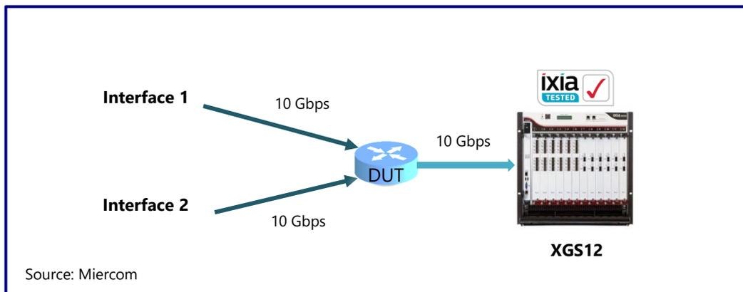
*The test topology for both tests was setup as shown above. Buffer was tested by sending traffic from two 10 GbE ports to one 10 GbE port with dynamic threshold and packet size of 64 to 9000 bytes.*
