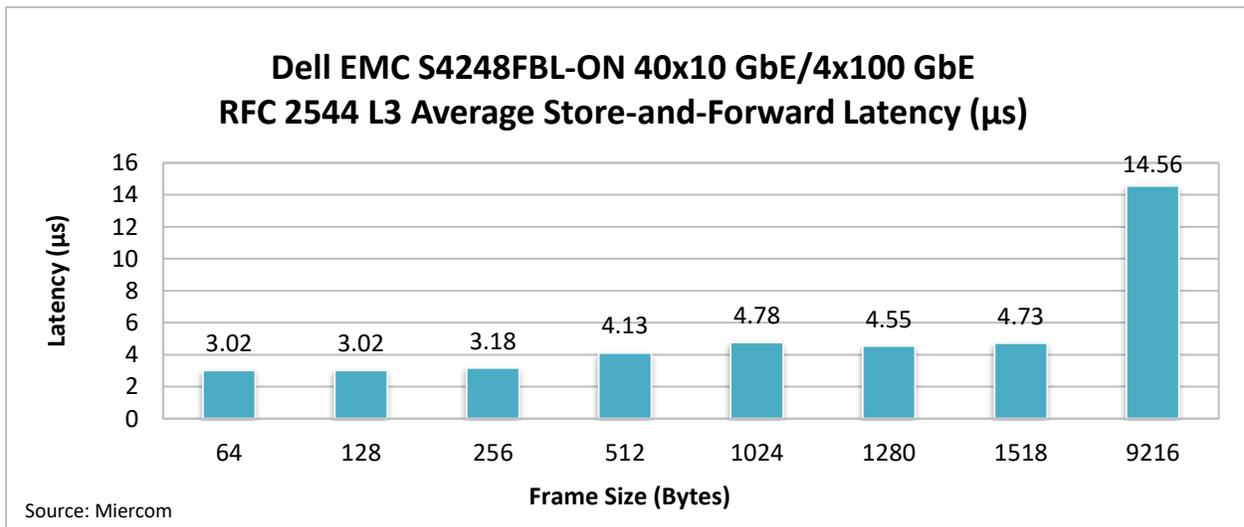
Lowest latency was observed for 64 and 128-byte frames, at 3.02 microseconds. Latency for all frame sizes remained under 14.56 microseconds. As expected, smaller frames were easier to process and had lower latency. The Dell EMC S4248FBL-ON switch was subjected to a 100-percent traffic load of Layer 3 unicast traffic on all 44 ports. Latency measurements were calculated in accordance with RFC 2544.
