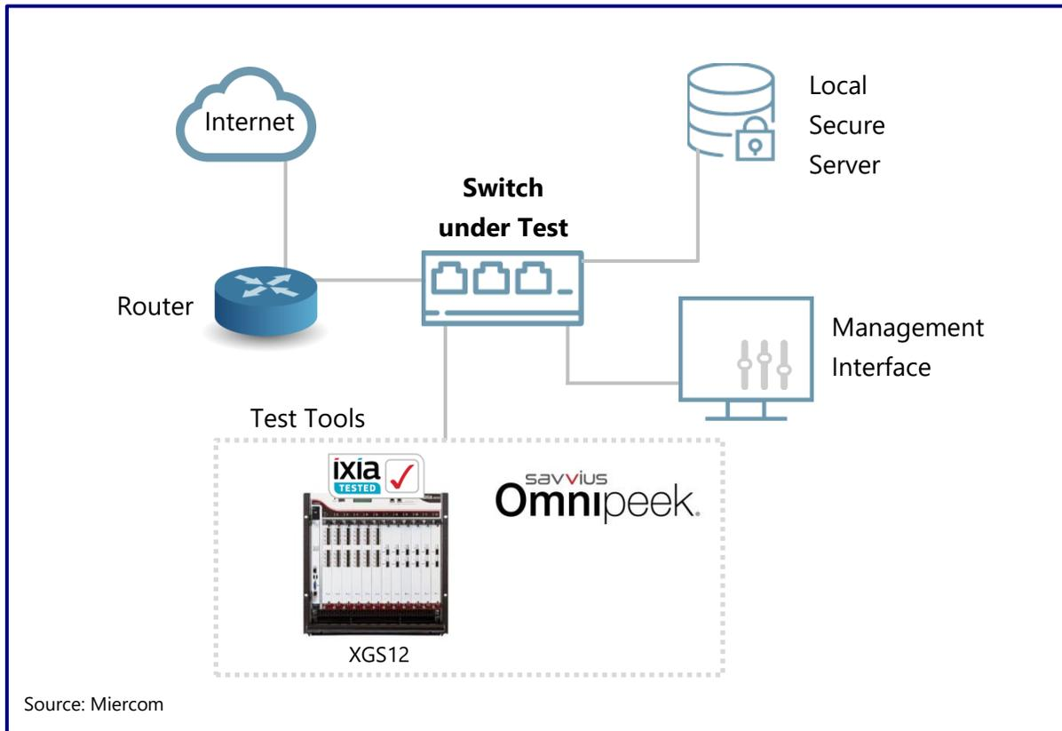
The Device Under Test (DUT) is deployed between the untrusted network from the Internet/switch and the local private network. The industry test tools are connected to the switch using 10 GbE and 100 GbE port pairs. The test tools generate traffic with different frame sizes, time intervals and device addresses to simulate a real-world data center environment.
