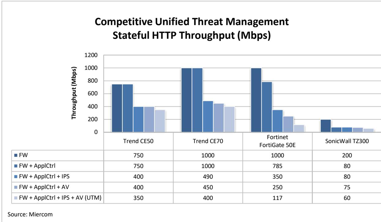
*Trend Micro CE70 had one of the highest firewall throughput rates of 1 Gbps, and UTM throughput of 400 Mbps. The Trend Micro CE50 had the second highest throughput rates for most configurations, and its UTM performance was nearly three times that of its next best competitor at 350 Mbps.*
