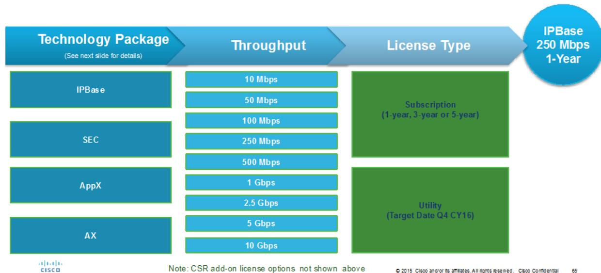
The CSR 1000V is licensed based on a combination of throughput and feature set. The package can be leased for a term of 1, 3 or 5 years or on a permanent, perpetual license.
