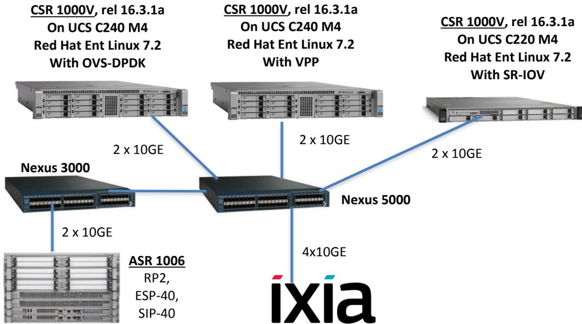
This test bed was used for all test cases on the Private Cloud. Each CSR1000V was configured for a different test in order to save configuration time.
