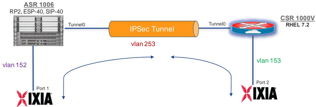
The CSR 1000V ran as a single virtual machine (VM), initially with a single vCPU configured. The I/O method used was SR-IOV (Single Root I/O Virtualization). RFC 2544 Throughput tests were then run.
