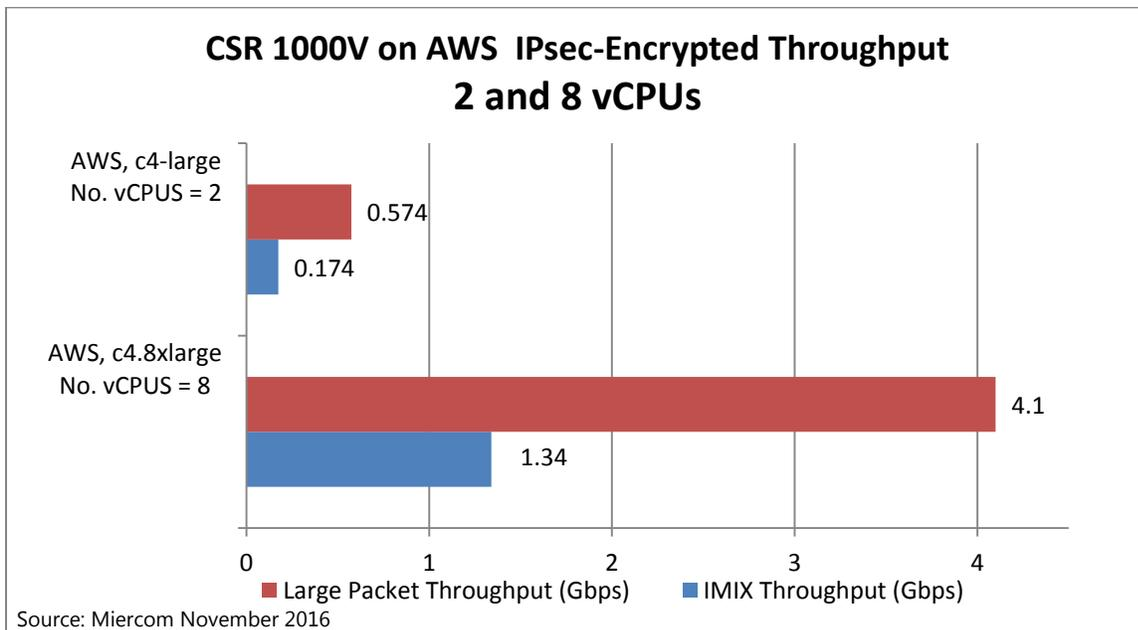
With full IPsec processing and encryption applied to all traffic through the IPsec tunnel, bi-directionally, 0.174 Gbps with IMIX traffic and 0.574 Gbps with large packet (1418 Bytes) traffic throughput was achieved in the AWS environment with a single vCPU. With eight vCPUs configured throughput climbed to 1.34 Gbps with IMIX traffic and 4.1 Gbps with large packet (1418 Bytes) traffic, about an eight-fold increase.
