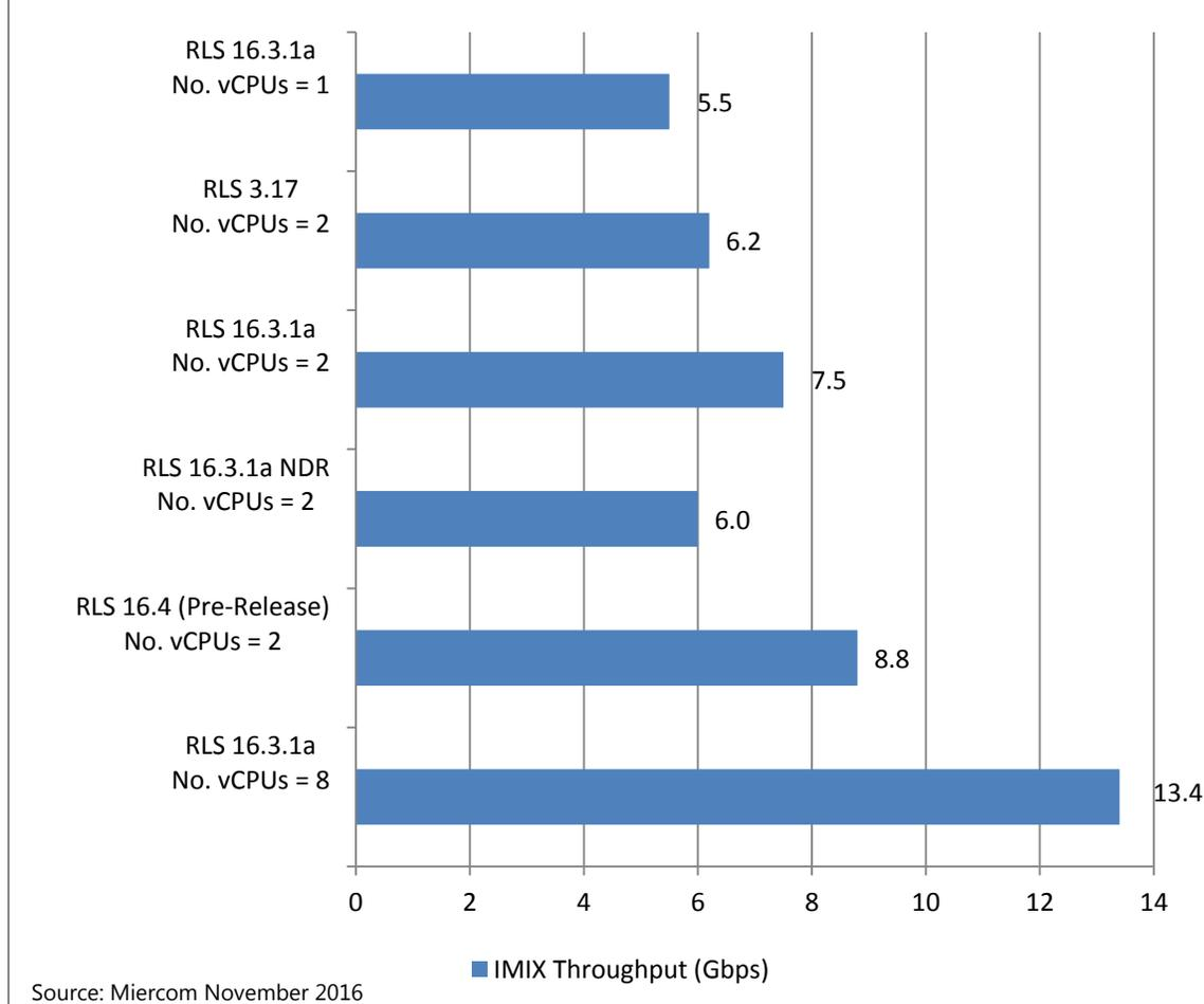
We also saw performance improvement by increasing the number of vCPUs. Where a single vCPU generated 5.5 Gbps of throughput, 13.4 Gbps could be achieved with eight vCPUs.
