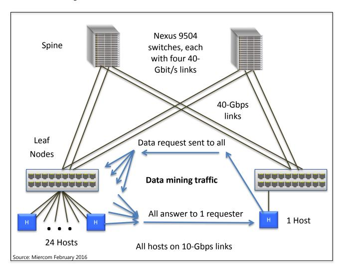
The test-bed data-center network featured two "spine" switches – Cisco Nexus 9504 modular switches. Each supported four 40-Gbps links to two "leaf" nodes, as indicated.
