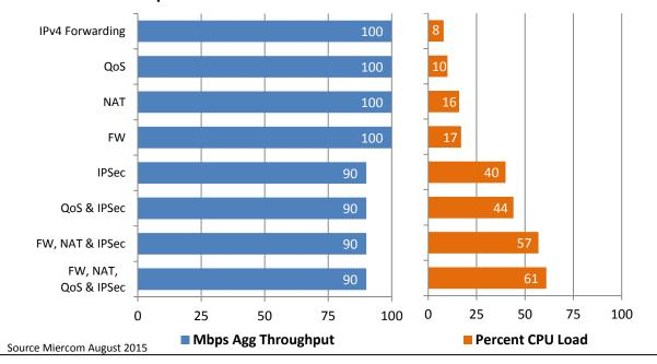
KEY: QoS = Hierarchical Quality of Service processing IPSec = All data is sent/received via encrypted tunnels
