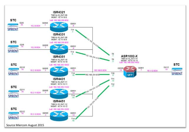
Test traffic was generated bidirectionally by the Spirent, at load levels set for the performance rating of each ISR 4000 model. Traffic was sent one-way directly from the STC test system to the ISR, which processed and forwarded the traffic onto and through a Cisco ASR1002-X, and then back to the return Spirent port. In the other direction, traffic was sent through the ASR1002-X, to the ISR, and back out to the return Spirent port, as shown in the diagram.
