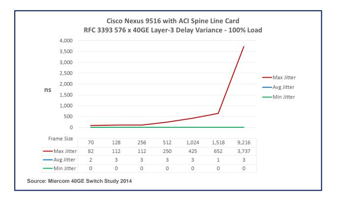
The Cisco Nexus 9516 exhibited very little variance in latency, also called "jitter" – less than 10 nanoseconds or less, on average, for all packet sizes up to 9,216-byte. The Cisco switch configured with 576 ports was subjected to a 100 percent traffic load. Layer-3 IP unicast traffic was used for the specified frame size. Tests were conducted in accordance with RFC 3393.
