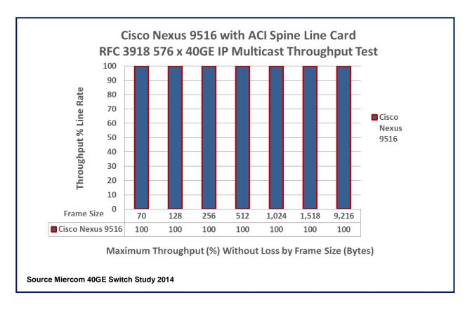
The Cisco Nexus 9516 with 16 x 36p 40G QSFP+ ACI spine line cards exhibits full-linerate multicast handling across all 576 of its 40GE ports, from a fully loaded input traffic stream. Tests were conducted in accordance with RFC 3918.
