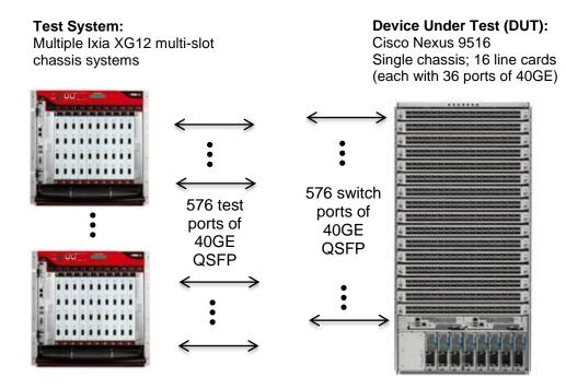
Actual Test Site: Shown below is the switch under test, surrounded by Ixia test systems.
