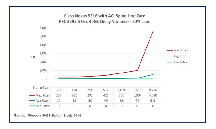
The Cisco Nexus 9516 exhibited very little variance in latency, also called "jitter" – less than 1 microsecond for all packet sizes up to 9,216-byte. The Cisco switch configured with 576 ports was subjected to a 50 percent traffic load. Layer-3 IP unicast traffic was used for the specified frame size. Tests were conducted in accordance with RFC 3393.
