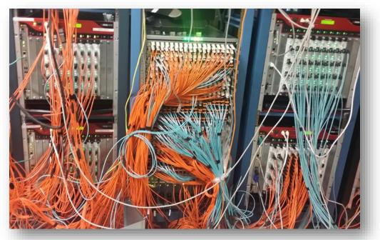
Once the array of Ixia XG12 tests systems were connected to the Nexus 9500, one Ixia system test port connected to each 40GE port on the switch, and connectivity confirmed on each port, we did not have to re-cable for the duration of the testing. The multiple chassis of the Ixia system are centrally controlled.
